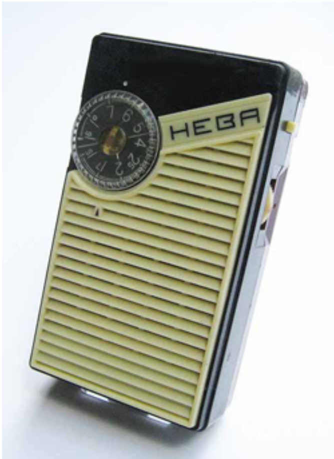
1960 Russia "Neva" (Нева): the first Soviet shirt pocket transistor radio, a six-transistor MW/LW radio manufactured at Radiopribor Factory, Leningrad (Saint Petersburg).
