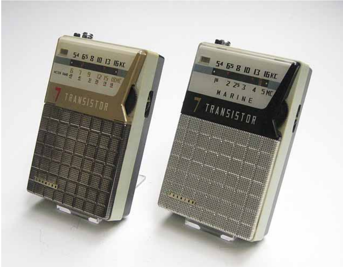
1960 TOSHIBA 7TP-352S, a 2-band, MW/SW pocket radio, its SW band covering 6 – 18 MHz; and its companion TOSHIBA 7TP-352M, covering MW and 1.6 – 5 MHz SW. Both radios have a seven-section 62mm telescopic antenna built into their cabinets. Other shirt pocket short wave transistor radios of the time included the Hitachi WH-761SB, the Jefferson-Travis JT-G200, the National T-21, and the Mitsubishi 7X-505.
