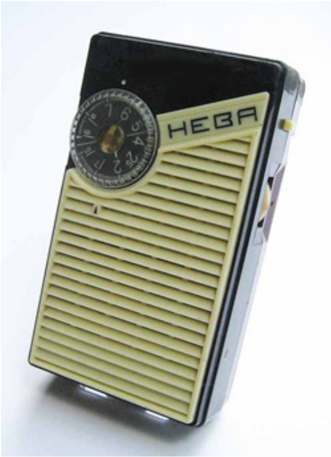
1960 Russia “Neva” (HeBa): the first Soviet shirt pocket transistor radio, a six-transistor MW/LW radio manufactured at Radiopribor Factory, Leningrad (Saint Petersburg).
