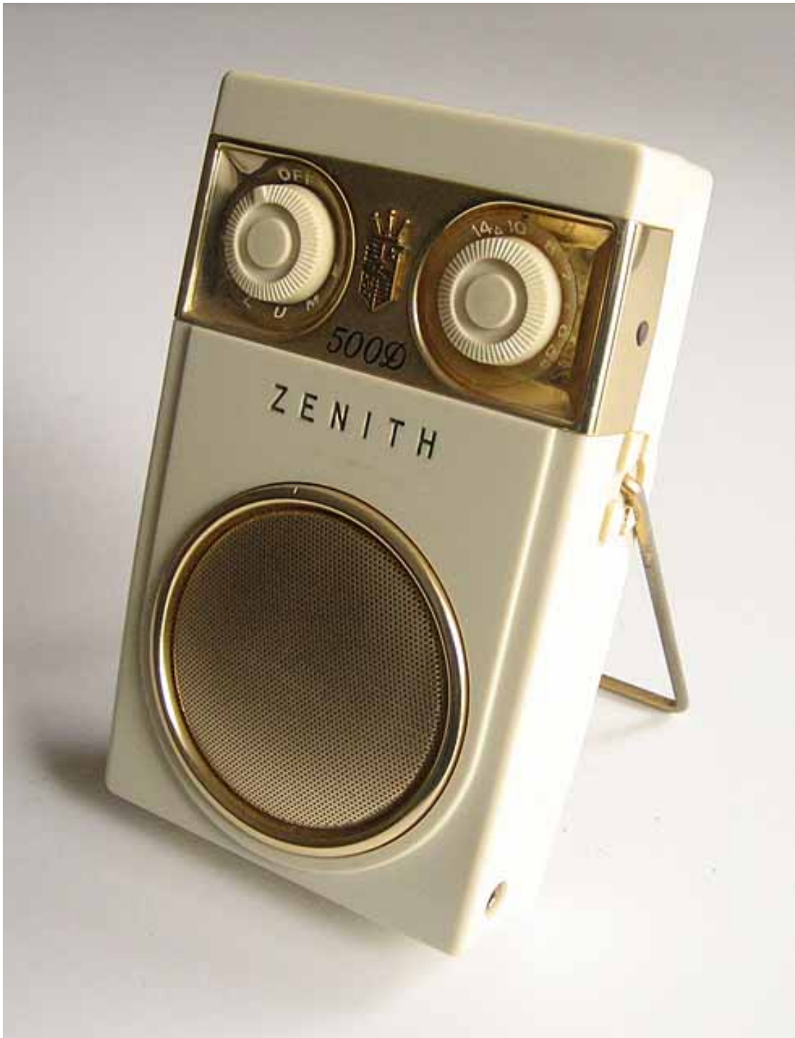
1959 ZENITH ROYAL 500D: a MW-only radio, like almost all US radios. The Zenith Royal 500 series was one of the most popular US transistor radios ever made, first produced in 1956 and continuing in production changes in cabinet design and circuit design over a long series of model numbers, culminating in the 1961 Zenith Royal 500H with a radical cabinet design change and more importantly its significantly enhanced AF and RF circuit designs and a large 3x5-inch speaker that would make it the best performing pocket transistor radio of its time.
