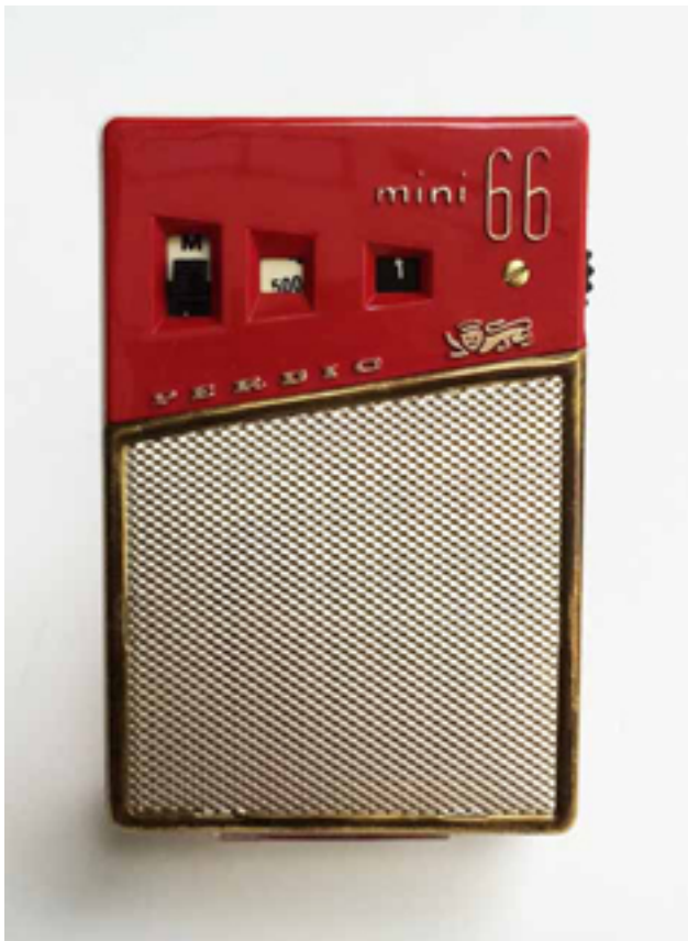
1962 Perdio PR33 “mini 66”: One of a very few shirt pocket transistor radio models made in Great Britain in the early 1960s – a two-band LW/MW radio, though its LW “band” was actually just a single pre-set frequency: 200 kHz (1500 meters), what was then BBC’s “Light Programme” station.
