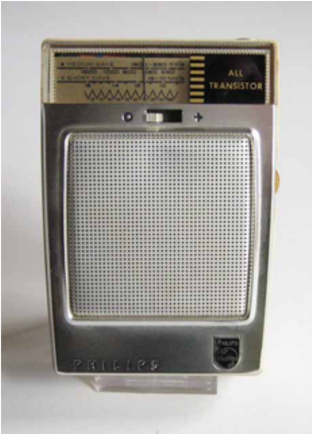
1963 PHILIPS L0X25T/22G: a 2-band, MW/SW pocket radio with a SW band covering 10 – 18 MHz
